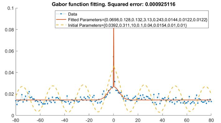
Fig. 3: Gabor function fitting with LM algorithm
