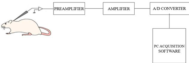
Fig. 1: **Acquisition chain:** Once the probe is inserted in the animal's brain, the neural signal picked up from the 32 contacts is transmitted to a preamplifier to remove noise contamination and further to an amplifier. Subsequently, it is digitized and managed by the acquisition software.
