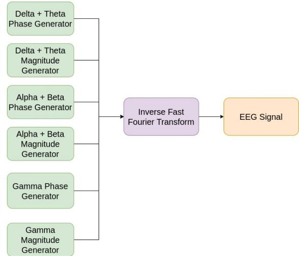
Fig. 2. Process of Reconstructing a Generated EEG Signal
