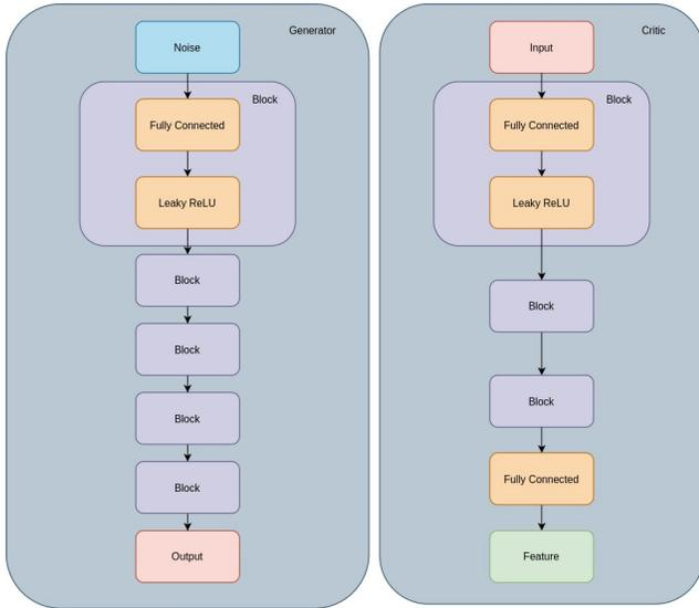
Fig. 1. Generator and Critic Architectures
